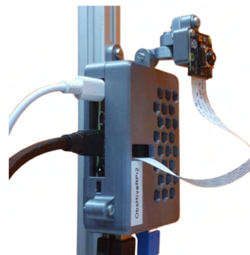
Figure 6: Camera and Raspberry Pi case (yaw, pitch and roll angles are adjustable).
